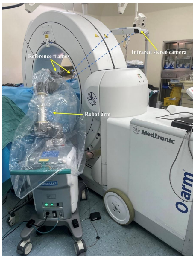
Fig. 3. TiRobot (TINAVI Medical Technologies Co. Ltd., Beijing, China) was used to assist the placement of upper cervical pedicle screws for treating atlantoaxial dislocation.
