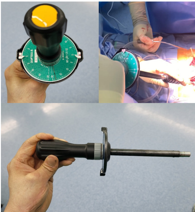
Fig. 1. The insertional torque was measured using a calibrated torque wrench with a specially designed connector for spine screw systems.
